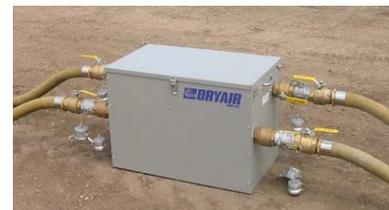
Figure 7 - Mixing/Booster Unit
