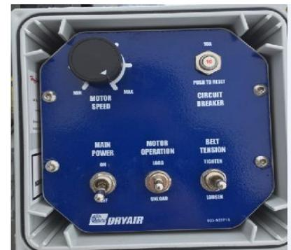
Figure 36 - Hose Reel Control Panel
