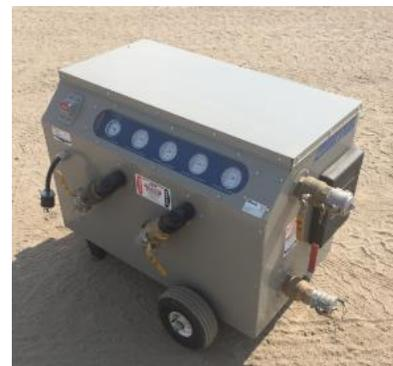
Figure 10 - Plate Heat Exchanger Unit
