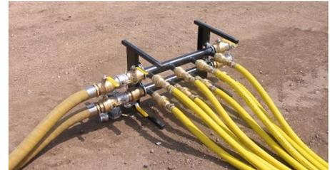
Figure 8 - Optional Remote Manifold
